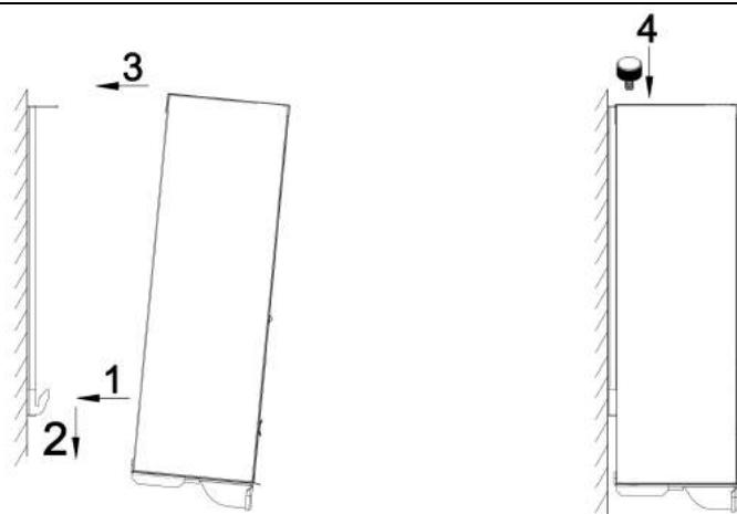
**STEP 3.** With the firebox at an angle, fit the slots in the back of firebox over the hooks on the wall mount bracket, and carefully press the top of the firebox against the wall mount bracket. The slots at the top edge of the firebox should slide over the wall mount bracket tabs. Hold the firebox in place and thread the thumb screws through the holes in the firebox and into the wall mount bracket tabs. Tighten both thumb screws and make sure the firebox is secure to the wall.
