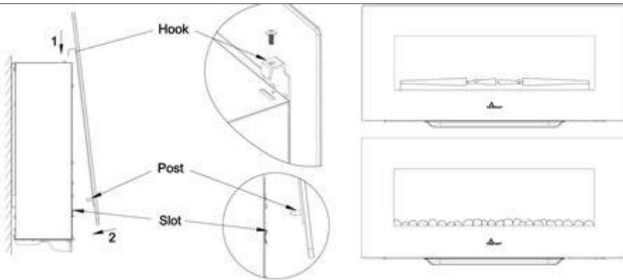
**STEP 6.** Carefully set both hooks of the front glass panel into the slots at the top front edge of the firebox. b. Press the two posts of the glass panel into the locking slots near the lower corners of the front firebox panel.
