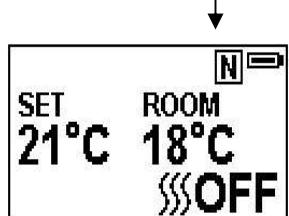
3.2.12 Press **SS A** button to turn on/off heat, **SS ON**, **SS OFF** will show at the lower of the screen.
