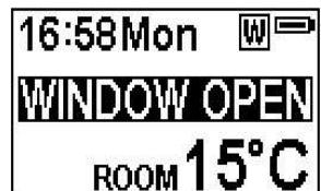
3.2.33 After the indoor temperature has risen or a manual override of the warning (by operating remote control) has been done, the fire will return to normal working state.
