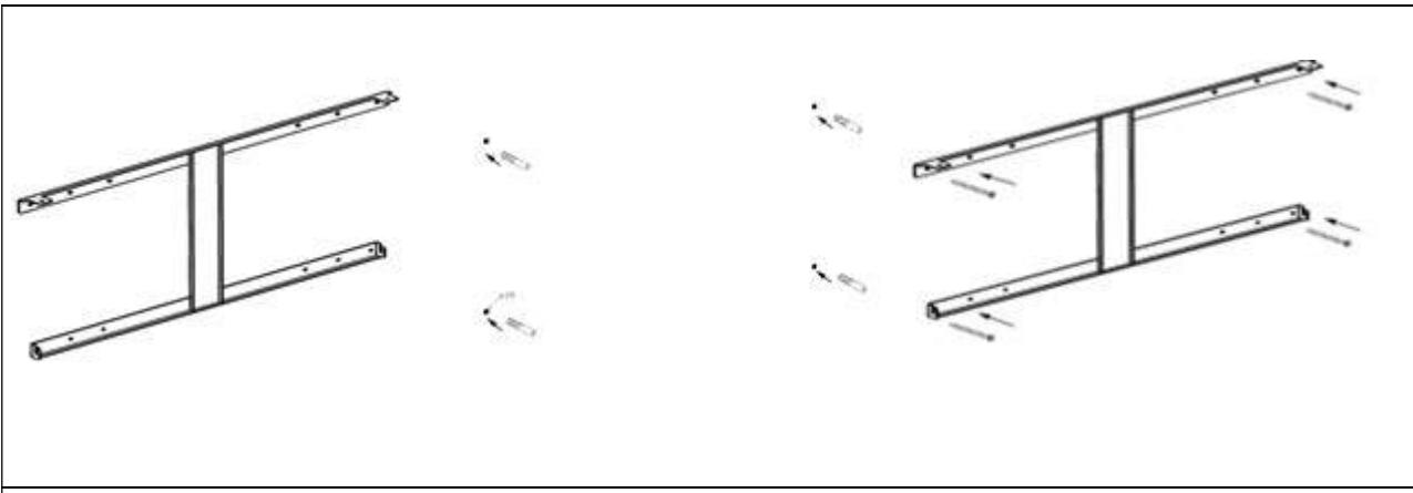
**STEP 2.** Choose a solid and plain wall and then put the bracket on the position where you want to install the fireplace. Mark the 4 holes by a pen from the holes on the bracket. Take away the bracket and then drill 4pcs  $\Phi 8$  holes on the wall. Put the plastic wall plug into the hole. If the wall is solid wood, it is no needed to drill the holes on the wood and no needed of the plastic wall plug. Then use 4pcs ST5\*40 to fix the bracket to the wall.
