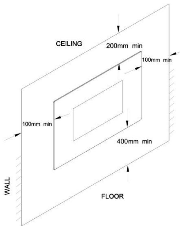
**STEP 1.** Find a safe location. Minimum clearance on each side must be at least 100mm; minimum clearance from the floor must be at least 66mm; minimum clearance from the front must be at least 3 feet (100 cm). Choose a location near an outlet so an extension cord is not required. **DO NOT** position the unit directly below a power outlet.
