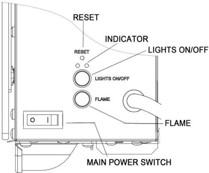
**NOTE: The manual button controls basic functions, not a full range of controls. Use the remote hand set to carry out all functions.** The manual buttons are located at the lower right corner of the appliance.
